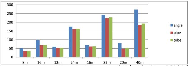
From these results it can be stated that the economic section is the tubular section which has both deflection and cost in the permissible limits
